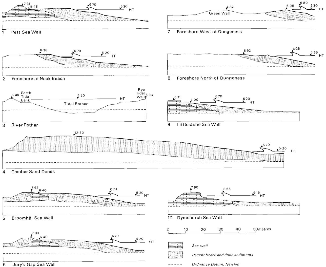
Fig. 13.2 Sea defences between Pett Level and Dymchurch. Sections show natural beach and dune profiles and sea walls. HT levels represent highest predicted astronomical tide for 300-year return period; associated maximum wave crest heights are also shown.
